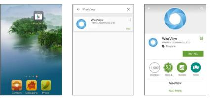
After installation, open WiseView and select "Device". Then click [ ] to add new device. Scan QR code under Information page. Then input client port, user name and password, and then click Save to log into the DVR.
